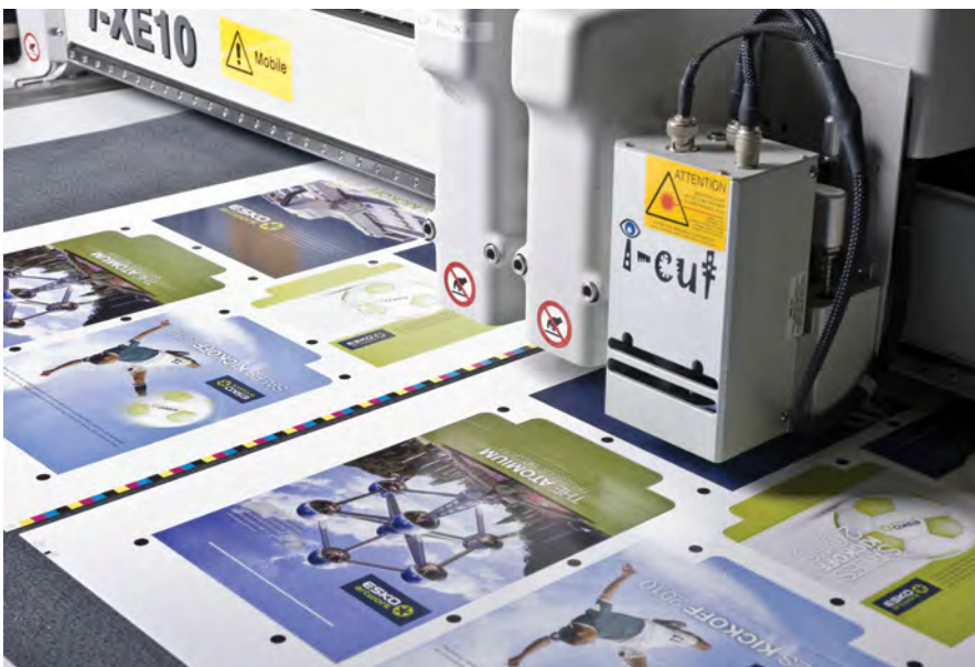
Figure 2: Esko's i-cut Suite is an automated PDF workflow for large-format printing. Use it to preflight files, optimize layouts, and create cutting paths and bleeds, and extend graphics.
