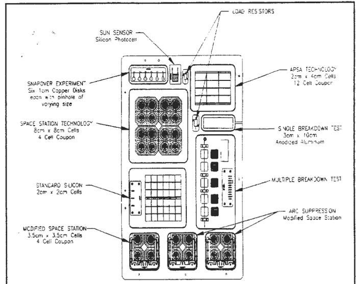
An experiment plate on top of the SAMPIE enclosure contains mounted samples of the different solar array cell technologies to be tested. The metal enclosure houses most of the measuring instruments, a data acquisition system, a power distribution system, and related electronics.
