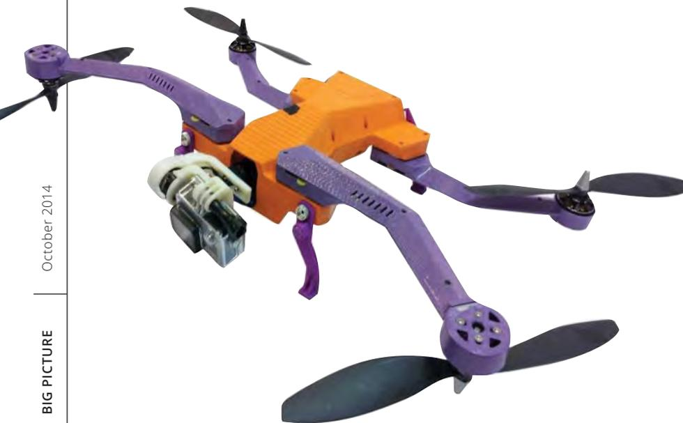
AirDog, the world's first automated drone designed to track and photograph outdoor sports and activities was made entirely from 3D-printed parts using the Stratasys' FDM technology. ([stratasys.com](http://stratasys.com))
